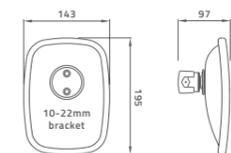
These versatile compact mirror heads can be used as rear view mirrors for Utility or small Agriculture vehicles, or as additional spotter mirrors on larger European style trucks. The 10-22mm bracket suitable version is particularly popular due to the mounting versatility.
